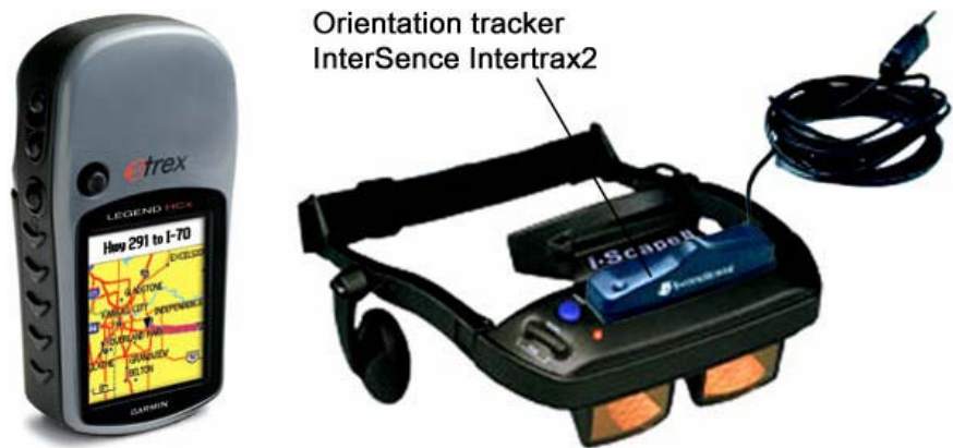
Figure 9 Garmin eTrex HCX GPS receiver and InterSense Intertrax2 fixed on Optical See-through Display (i-Glasses- Scape II HMD)
